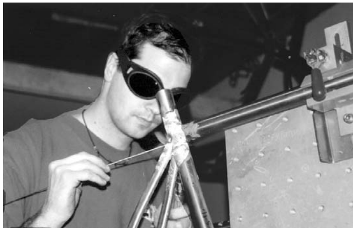
STEEL LIFE—Frame builder Chris Zanotti fillet-brazes a top tube to a seat junction on one of his hand-crafted steel frames.
